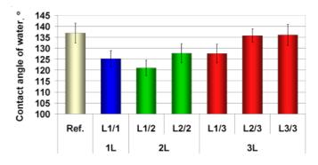
**Figure 7.** Contact angles of argon plasma treated nonwoven layers (L), measured two weeks after the treatments.
