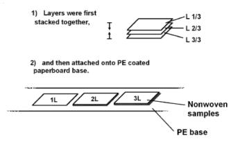
Figure 3. Sample preparation for plasma treatments in a continuous line.
