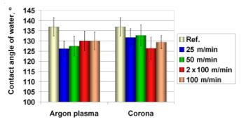
Figure 10. Contact angles of nonwoven samples treated with different speeds / exposure times, measured one week after treatments.
