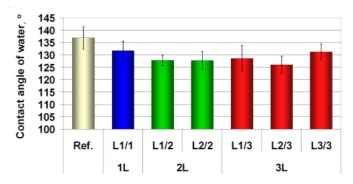
Figure 8. Contact angles of corona treated nonwoven layers (L), measured two weeks after the treatments.
