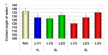
Figure 6. Contact angles of helium plasma treated nonwoven layers (L), measured two weeks after the treatments.
