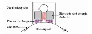
**Figure 4.** An atmospheric plasma treatment unit in operation (top) and a simplified sketch of an atmospheric plasma treatment unit (bottom).
