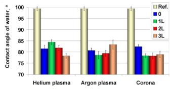
Figure 9. Contact angles of the base material surface (PE-LD) after the plasma and corona treatments measured from below different numbers of nonwoven layers (0-3 L), measured one day after the treatments.
