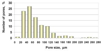
Figure 5. Pore size distribution of the nonwoven.
