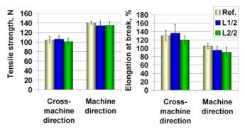
**Figure 12.** Maximum breaking strength and elongation of the test piece at the maximum breaking strength: argon plasma treated nonwoven layers (two-layered sample).
